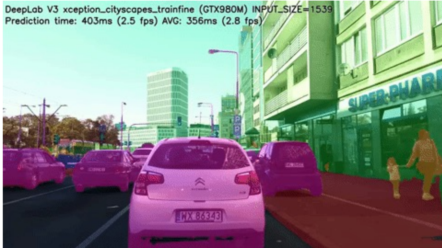
A real-time segmented road scene for autonomous driving
